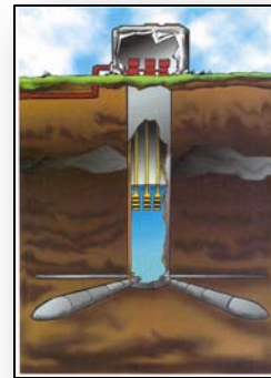
Figure 7.1: Example of a Radial Collector Well
