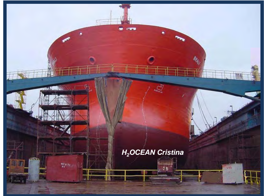
48,000 DWT tanker; 182 meters long by 32 meters wide by 18 meters deep
